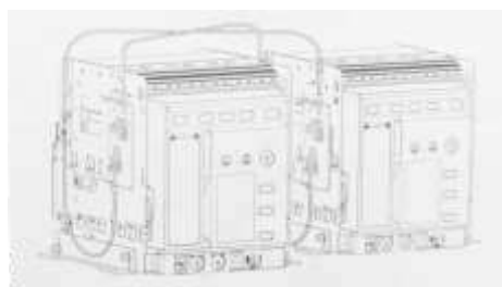
Mechanical Interlock using Bowden Cable
